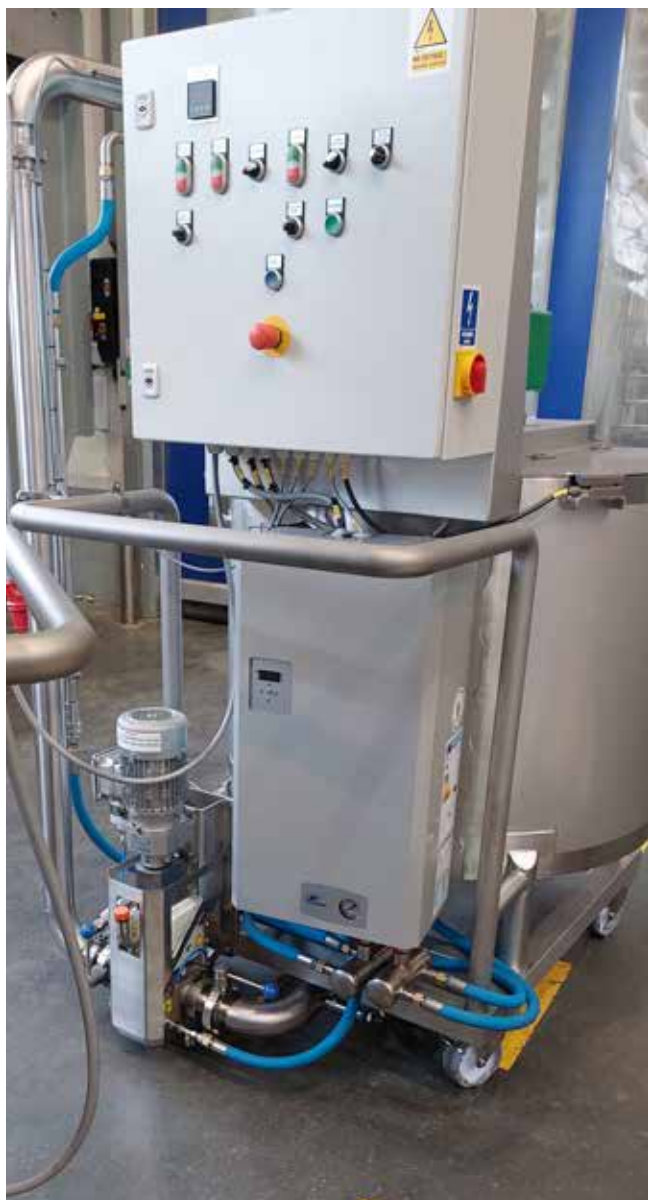
Pumped liquid - cookie fillings, confectionery products Pump - LPX80-1 with heated cover, installed vertically to save space
