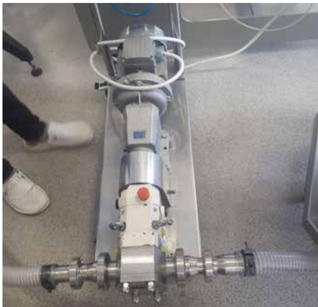
Pumped liquid - toothpaste, body scrubs, lotions creams Pump - LPX50-1 delivering 2 m 3 /h at 5 bar differential pressure
