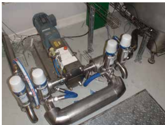
Pumped liquid - glucose Syrup 80 °Bx Pump - LPX50-1 with heated cover and double mechanical seal
